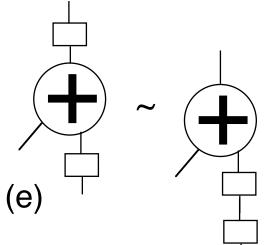
Noise gates may be "moved along wires and thru any other gates"
