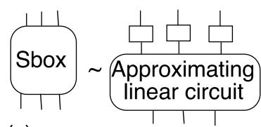
(c) Any Sbox may be replaced by this equivalent circuit
